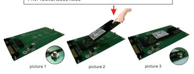
Step 1: Put copper nut on the same side of the NGFF connector; and fix M3x5mm screw from bottom to top of the adapter(picture 1).
